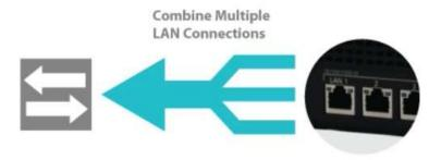
Use 802.3ad to combine multiple LAN connections into a virtual LAN connection. This virtual connection has higher throughput and redundancy in case any single link fails.
