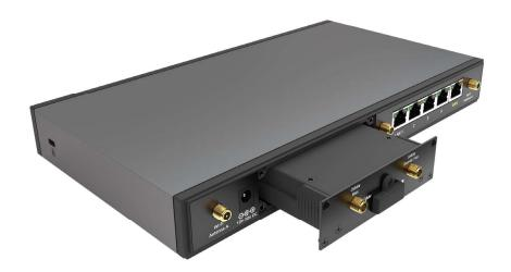
Step 3: Screw on the screw and fix the module.
