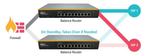
When your organization has a corporate requirement demanding the highest availability with no single point of failure, you can deploy two Peplink routers in <u>High Availability mode</u>. With High Availability mode, the second device will take over when needed.
