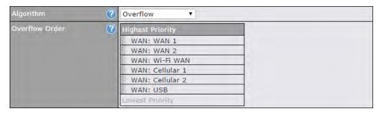
Drag and drop to specify the order of WAN connections to be used for routing traffic. Only the highest priority healthy connection that is not in full load will be used.
