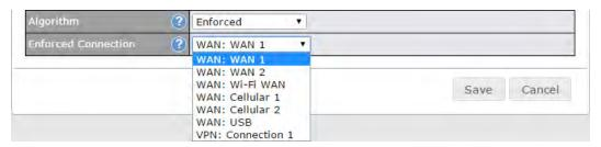
Matching traffic will be routed through the specified WAN connection, regardless of the health check status of the WAN connection. Starting from Firmware 5.2, outbound traffic can be enforced to go through a specified SpeedFusion<sup>™</sup> connection.
