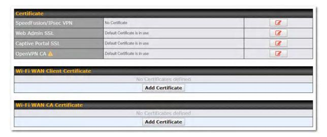
This section allows for certificates to be assigned to the local VPN, Web Admin SSL, Captive Portal SSL, OpenVPN CA, Wi-Fi WAN Client certificate and Wi-Fi WAN CA Certificate.
