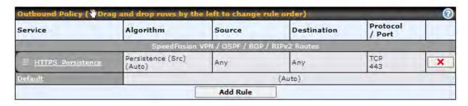
The bottom-most rule is **Default**. Edit this rule to change the device's default manner of controlling outbound traffic for all connections that do not match any of the rules above it. Under the **Service** heading, click **Default** to change these settings.
