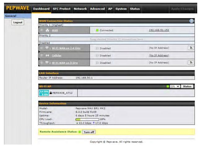
The **Dashboard** shows current WAN, LAN, and Wi-Fi AP statuses. Here, you can change WAN connection priority and switch on/off the Wi-Fi AP. For further information on setting up these connections, please refer to **Sections 8** and **9**.
