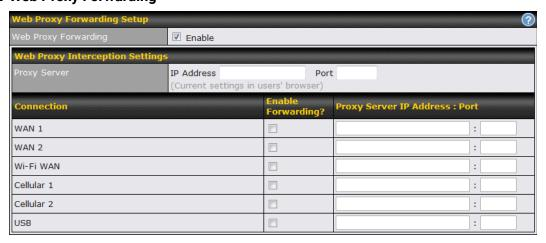
When this feature is enabled, the Pepwave router will intercept all outgoing connections destined for the proxy server specified in **Web Proxy Interception Settings**, choose a WAN connection with reference to the outbound policy, and then forward them to the specified web proxy server and port number. Redirected server settings for each WAN can be set here. If forwarding is disabled for a WAN, web proxy connections for the WAN will be simply forwarded to the connection's original destination.
