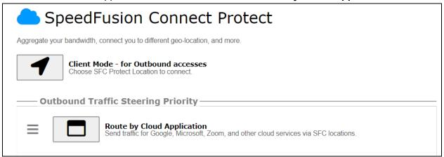
Select a Cloud application to route through SpeedFusion Connect Protect from the drop down list > Click > Save > Apply Changes.
