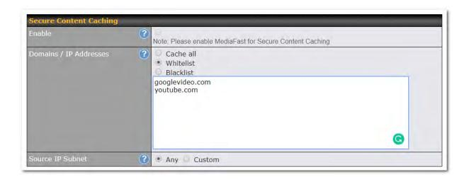
The **Secure Content Caching** menu operates identically to the **MediaFast** menu, except it is for secure content cachting accessible through https://.
