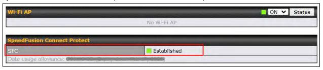
If you are running a latency sensitive service like video streaming or VOIP, a WAN Smoothing sub-tunnel can be created. Navigate to Navigate to SFC Protect > Client Mode - for Outbound accesses > SFC.
