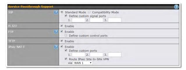
Some Internet services need to be specially handled in a multi-WAN environment. Pepwave routers can handle these services such that Internet applications do not notice being behind a multi-WAN router. Settings for service passthrough support are available here.
