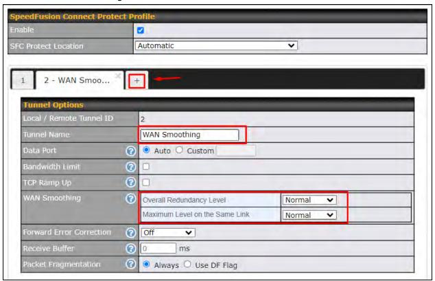
Click on **Save** and **Apply Changes** to save the configuration. Now, the router has 2 Speedfusion tunnels to the SpeedFusion Connect Protect.
