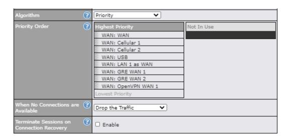
Starting from Firmware 5.2, outbound traffic can be prioritized to go through SpeedFusion<sup>™</sup> connection(s). By default, VPN connections are not included in the priority list.
