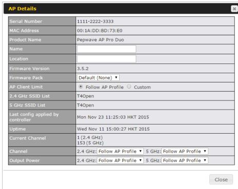
For easier network management, you can give each client a name and designate its location. You can also designate which firmware pack (if any) this client will follow, as well as the channels on which the client will broadcast.
