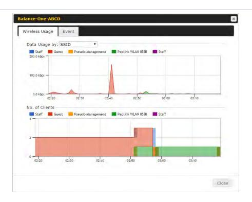
Click any point in the graphs to display detailed usage and client information for that device, using that SSID, at that point in time. On the **Data Usage by** menu, you can display the information by SSID or by AP send/receive rate.
