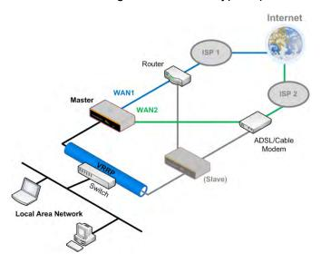
In the diagram, the WAN ports of each Pepwave router connect to the router and to the modem. Both Pepwave routers connect to the same LAN switch via a LAN port.
