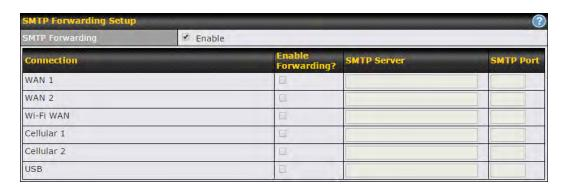
To enable the feature, select **Enable** under **SMTP Forwarding Setup**. Check **Enable Forwarding** for the WAN connection(s) that needs forwarding. Under **SMTP Server**, enter the ISP's e-mail server host name or IP address. Under **SMTP Port**, enter the TCP port number for each WAN.
