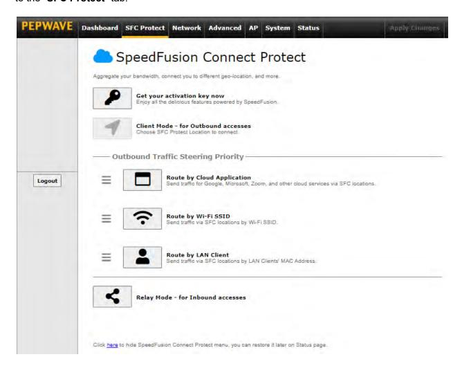
To setup a Peplink Relay Mode, select "Relay Mode - for Inbound accesses" > Choose the SFC Protect Location you wish to connect to > Click on the Green tick button to confirm the change.
