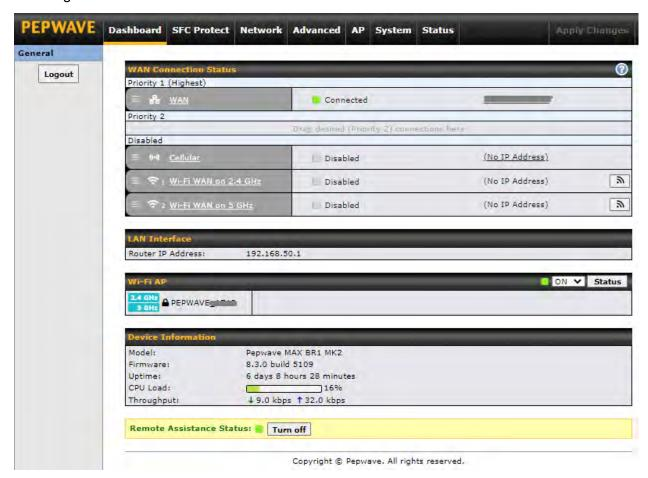
To able a particular WAN connection, drag on the appropriate WAN by holding the left mouse button, move it the **Disabled** row, and drop it by releasing the mouse button.
