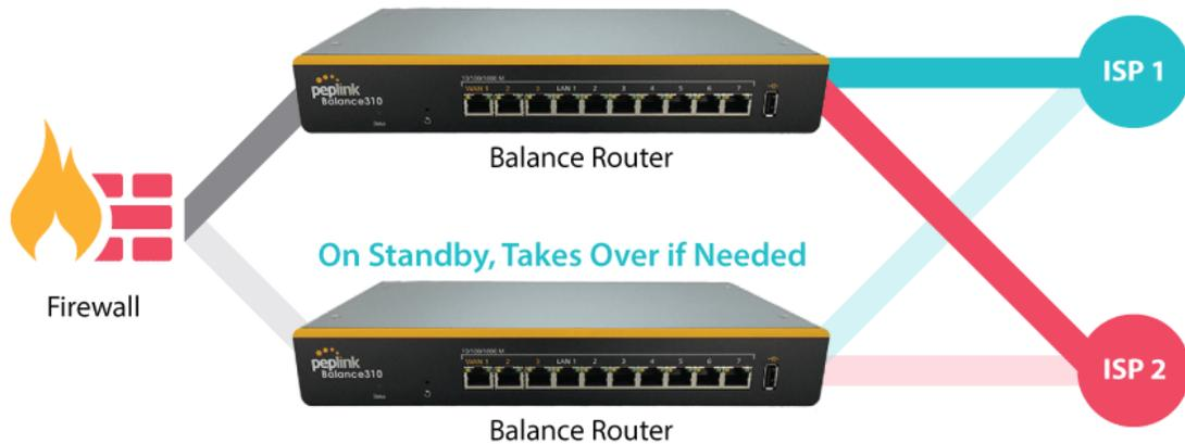
When your organization has a corporate requirement demanding the highest availability with no single point of failure, you can deploy two Peplink routers in [High Availability mode](#). With High Availability mode, the second device will take over when needed.
