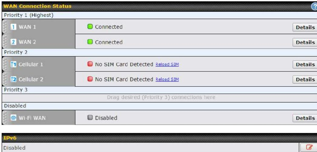
To enable a particular WAN connection, drag on the appropriate WAN by holding the left mouse button, move it to the **Disabled** row, and drop it by releasing the mouse button.
