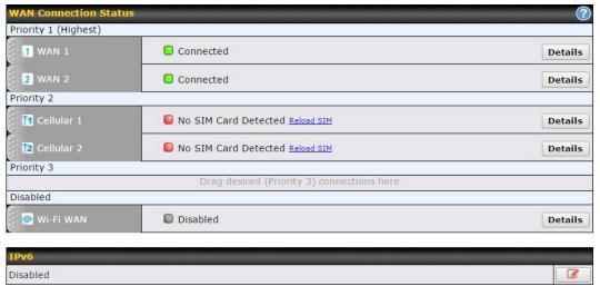
To disable a particular WAN connection, drag on the appropriate WAN by holding the left mouse button, move it the **Disabled** row, and drop it by releasing the mouse button. You can also set priorities on the **Dashboard**. Click the **Details** button in the corresponding row to modify the connection setting.
