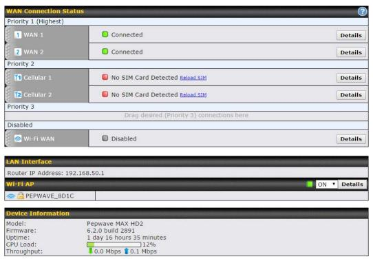
The **Dashboard** shows current WAN, LAN, and Wi-Fi AP statuses. Here, you can change WAN connection priority and switch on/off the Wi-Fi AP. For further information on setting up these connections, please refer to **Sections 8** and **9**.
