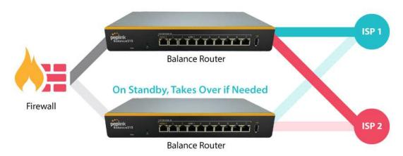
When your organization has a corporate requirement demanding the highest availability with no single point of failure, you can deploy two Peplink routers in **High Availability mode**. With High Availability mode, the second device will take over when needed.
