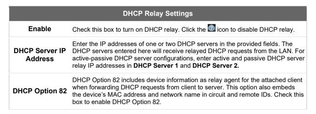
Once DHCP is set up, configure LAN Physical Settings, Static Route Settings, WINS Server Settings, and DNS Proxy Settings as noted above.
