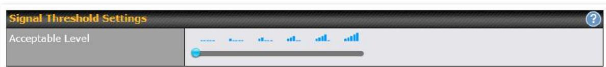
If signal threshold is defined, this connection will be treated as down when a weaker than threshold signal is determined.
