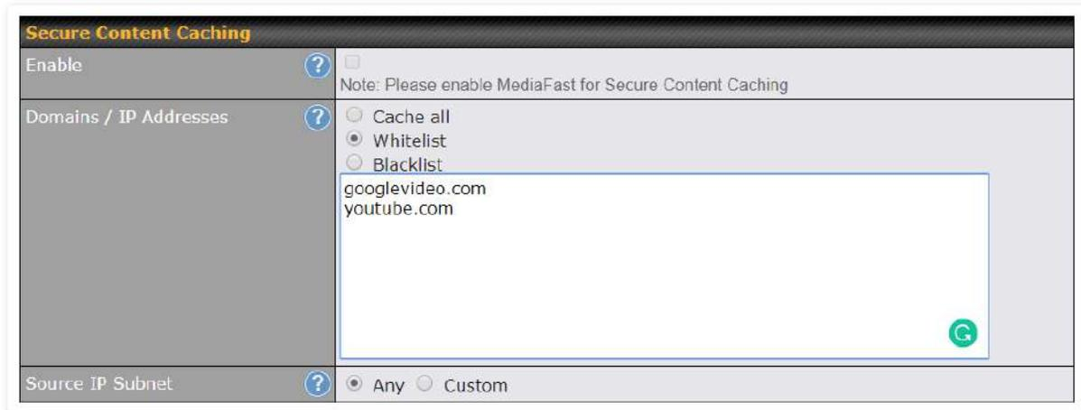
The **Secure Content Caching** menu operates identically to the **MediaFast** menu, except it is for secure content caching accessible through https://. In order for Mediafast devices to cache and deliver HTTPS content, every client needs to have the necessary certificates installed\*.
