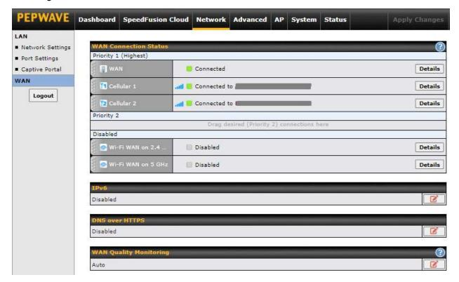
To able a particular WAN connection, drag on the appropriate WAN by holding the left mouse button, move it the **Disabled** row, and drop it by releasing the mouse button.
