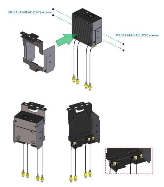
STEP 3: Assemble SMA connectors to the bracket
