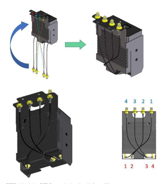
STEP 4: Lock the SFE-Duo set in the slot with 2 pcs M3 screws.
