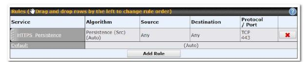
The bottom-most rule is **Default**. Edit this rule to change the device's default manner of controlling outbound traffic for all connections that do not match any of the rules above it. Under the **Service** heading, click **Default** to change these settings.
