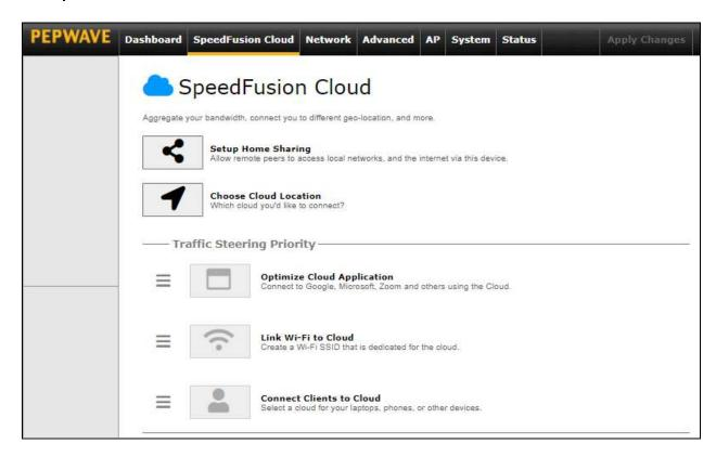
To setup a SpeedFusion Cloud Relay Server, select "Setup Home Sharing" > Choose the Cloud Location you wish to connect to > Click on the green tick button to confirm the change.
