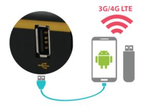
For increased WAN diversity, plug in a USB LTE modem as a backup. Peplink routers are compatible with over <u>200 modem types</u>. You can also tether to smartphones running Android 4.1.X and above.
