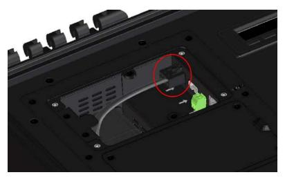
• STEP 3: Lock the slot cover with 4 pcs M3 screws.
