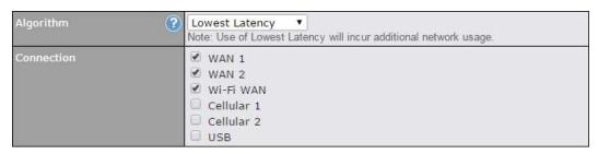
The traffic matching this rule will be routed through the healthy WAN connection that is selected in **Connection** and has the lowest latency. Latency checking packets are issued periodically to a nearby router of each WAN connection to determine its latency value. The latency of a WAN is the packet round trip time of the WAN connection. Additional network usage may be incurred as a result.
