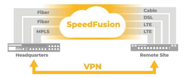
Pepwave bandwidth bonding SpeedFusion<sup>™</sup> is our patented technology that enables our SD-WAN routers to bond multiple Internet connections to increase site-to-site bandwidth and reliability. SpeedFusion functionality securely connects your Pepwave router to another Pepwave or Peplink device (Peplink Balance 210/310/380/580/710/1350 only). Data, voice, or video communications between these locations are kept confidential across the public Internet.
