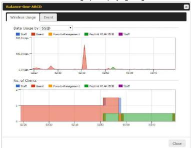
Click any point in the graphs to display detailed usage and client information for that device, using that SSID, at that point in time. On the **Data Usage by** menu, you can display the information by SSID or by AP send/receive rate.
