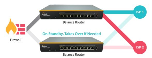
When your organization has a corporate requirement demanding the highest availability with no single point of failure, you can deploy two Peplink routers in <a href="High Availability mode">High Availability mode</a>. With High Availability mode, the second device will take over when needed.
