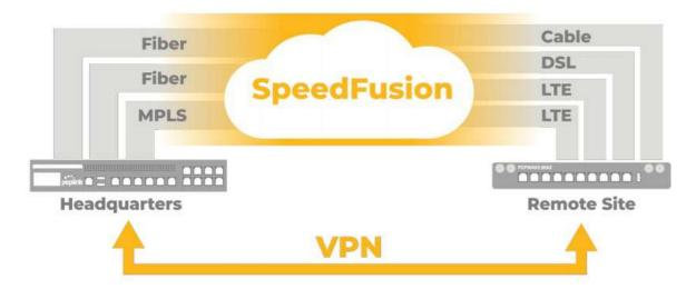
Pepwave bandwidth bonding SpeedFusion<sup>TM</sup> is our patented technology that enables our SD-WAN routers to bond multiple Internet connections to increase site-to-site bandwidth and reliability. SpeedFusion functionality securely connects your Pepwave router to another Pepwave or Peplink device (Peplink Balance 210/310/380/580/710/1350 only). Data, voice, or video communications between these locations are kept confidential across the public Internet.
