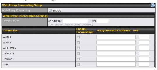
When this feature is enabled, the Pepwave router will intercept all outgoing connections destined for the proxy server specified in **Web Proxy Interception Settings**, choose a WAN connection with reference to the outbound policy, and then forward them to the specified web proxy server and port number. Redirected server settings for each WAN can be set here. If forwarding is disabled for a WAN, web proxy connections for the WAN will be simply forwarded
