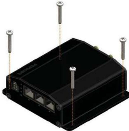
For type 2, the device requires two screws for wall mounting.
