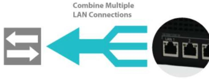
Use 802.3ad to combine multiple LAN connections into a virtual LAN connection. This virtual connection has higher throughput and redundancy in case any single link fails.
