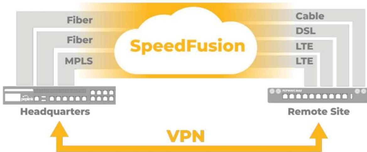
Peplink Balance SpeedFusion™ Bandwidth Bonding is our patented technology that enables our SD-WAN routers to bond multiple Internet connections to increase site-to-site bandwidth and reliability. SpeedFusion securely connects one or more branch offices to your company's main headquarters or to other branches. The data, voice, and video communications between these locations are kept confidential across the public Internet.
