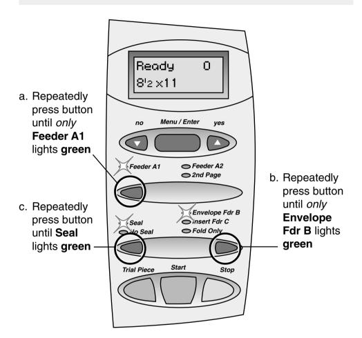
A **green** indicator shows that a feeder or function is selected. Repeatedly pressing the selection buttons (a, b and c above)
