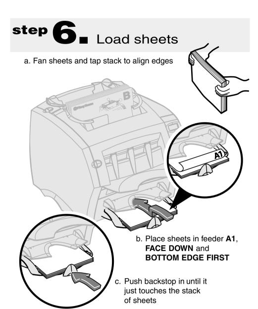
Use test sheets marked with **A1**. Use Sheet Feeder **A1** for sheets that need folding.
