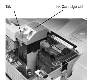
2. Push the tab on the front of the cartridge lid. Lift the lid up and push toward the back of the machine.
