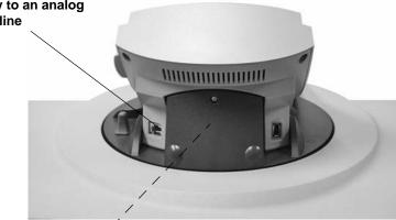
IntelliLink® Control Center installed on a DM1100<sup>™</sup> Digital Mailing System base. Dotted line indicates AC Adapter Receptacle is covered by base
