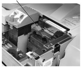
5. Push the printhead tab to the left. While continuing to press the printhead tab to the left, pull the assembly forward as shown here.
