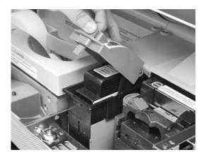
Remove the old ink cartridge by lifting it straight up.
