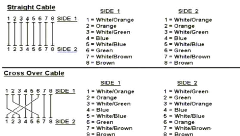
Figure A-1: Straight-Through and Crossover Cable
