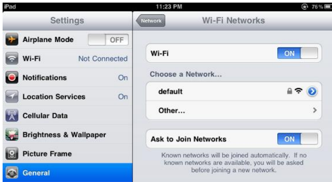
Figure 6-20 Turn on Wi-Fi
