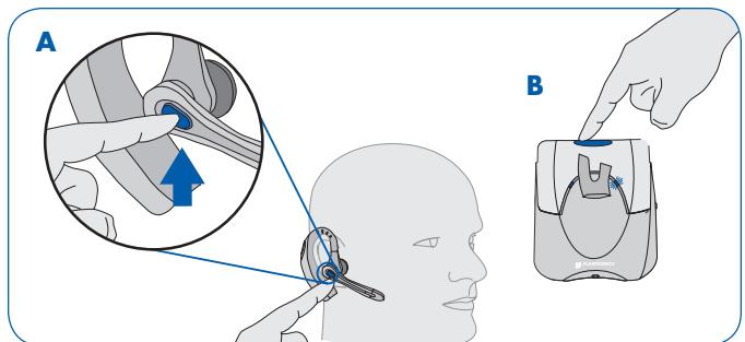
**US** If either the mobile handset or corded telephone are ringing, then press the Call Control button on either the headset (**A**) or base (**B**) to answer the call.
