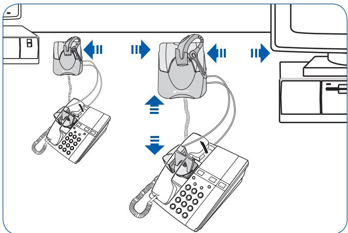
**US** Positioning: Recommended separation distance. **Important:** Incorrect positioning can cause problems with noise and interference.
