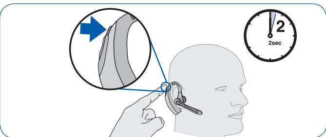
**US** To turn the headset on, press in and hold the Power/Mute Button for 2 seconds until the Status Indicator flashes blue. To turn off, press and hold the button again for 2 seconds until the Status Indicator flashes red.
