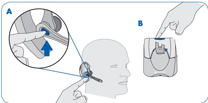
**US Placing a call on your corded telephone:** Lift the handset and then press either the Call Control button on the headset (**A**) or base unit (**B**). When you hear the dial tone, dial as normal. If you do not obtain a dial tone, check that the Configuration Dial is set correctly as described on page 11.
