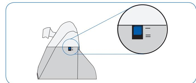
**US** When the L510S Bluetooth Wireless Headset System is used in conjunction with a Plantronics Handset lifter, you can enable the IntelliStand™ feature.
