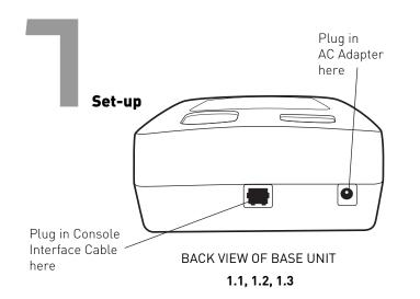
**1.1** Set up the CA12CD Amplifier as shown.
