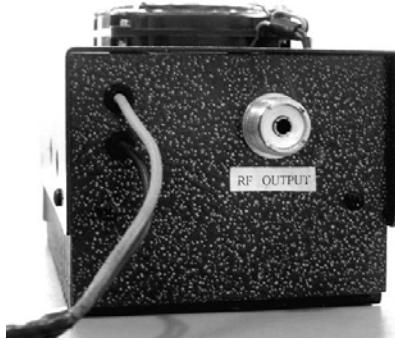
4. Connect the negative power wire on the back of the OM-1 to the negative side of a 13.8 volt power supply.
