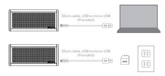
When charging is complete, the Power LED will stop flashing and illuminate solid if The Blaster is already powered ON, or turn off completely if The Blaster is powered OFF.
