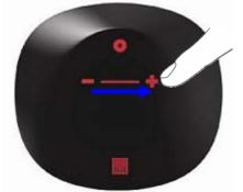
• Slide from **"Left to Right" on the Volume buttons** for rejecting the call (When the phone is ringing)
