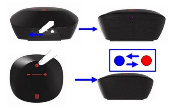
• Press and hold "**Multi-Function**" Button until the front Grid flashing in BLUE/RED, and the Speaker will says "Discovering"; PF309 has 3 mins (searchable time) for your BT device to pair with.
