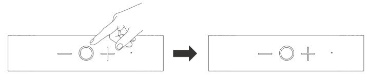
2) Hold down the "MFB" until LED flashing Blue + Red and connect to your Bluetooth device
