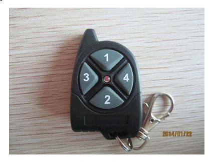
This remote control is used to work with receiver. Remote control is to transmit signal and receiver is to receive signal. No other usage.
