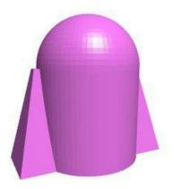
When finished, render the shape and generate the STL file for your printer. While you can make any size robot you wish, I made mine 90 mm high, with a radius of 30 mm.
