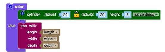
When this BlocksCAD program is run, it produces the following tree. I changed the rendering color by clicking on the Render window box with the color swatch and choosing green as the new color since it looks more treelike. Of course the color of your printed object will be determined by the filament you use.
