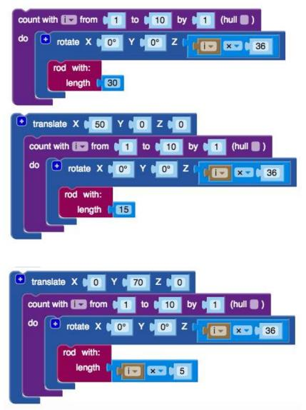
The third shape uses "i" as a variable as part of the calculation for the rod length, showing that you can use variables, not just numbers, in your modules.
