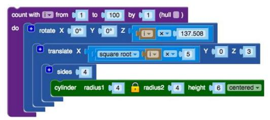
This instruction set puts 100 seeds on the disk. Each seed is made from a quadrilateral using a cylinder with four sides. Each seed is positioned along the X-axis by the square root of the count value (i) so they will be pretty evenly spaced along the radius of the disk. This number is multiplied by 5 to keep the seeds from overlapping. The translated seed is then rotated around the Z-axis by our Golden Angle times the index value.
