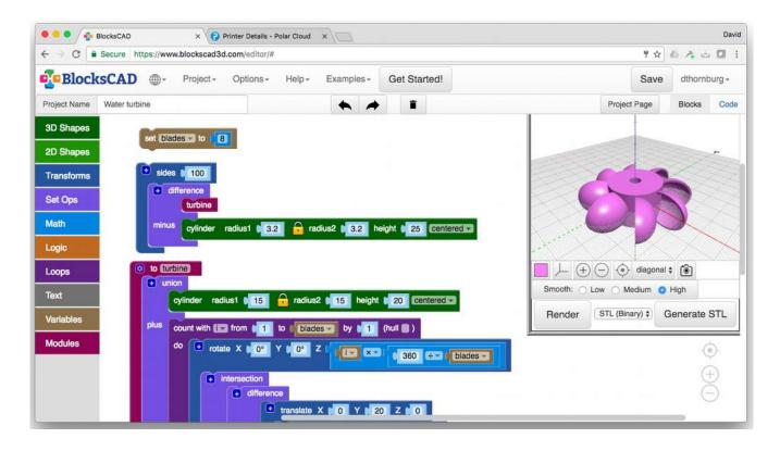
There are ten color-coded buttons representing block categories on the left side of the screen. Each of these categories brings up the different kinds of objects used in a BlocksCAD program. These include two kinds of shapes (both 3D and 2D), various transformations, setting different operations on our shapes, math operations, logic operations, loops, text, variables, and the definition and use of modules you can build to collapse large program segments you use over again into a single command.
