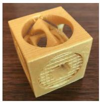
The support structures are holding the three cubes together. You can peel the supports away with needle nose pliers and dental picks, allowing the three cubes to wiggle around the structure independently.
