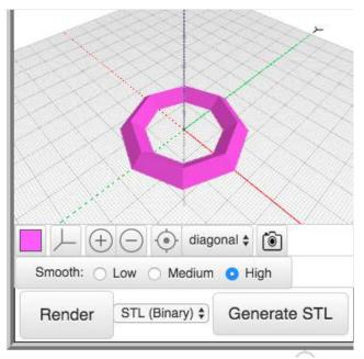
Now let's look at the parameters for this shape. Radius1 is the radius of the torus itself — the distance from the origin to the center of the shape along the X-axis. Radius2 is the radius of the tube itself. Sides represent the number of sides in our ring (in our case, 8). Faces represent the number of faces in the tube itself — in our case, 4.
