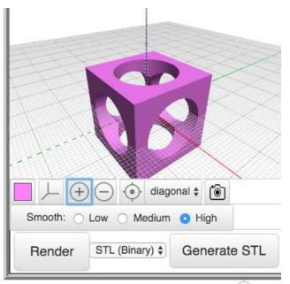
Unlike the Union operation, this one works a bit differently. The first shape in the list is the object from which the remaining shapes are subtracted. If you add more spaces for items to subtract than you need, you can remove them (starting at the bottom of the block) by clicking on the – (minus) sign at the top of the block.
