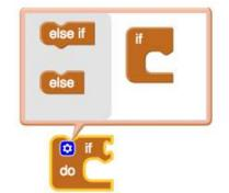
The most common modification is the addition of the Else command created by dragging the Else block inside the If block in the upper window. Once it is in place, click on the gear to collapse the modification window.
