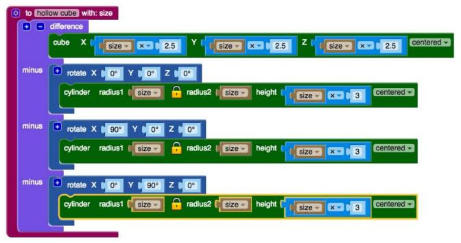
Next, we draw three of them with different sizes. The middle one is rotated around the Z-axis by 45° so everything just fits. The sizes were chosen so that, when finished, each hollow cube is not touching either of the others.
