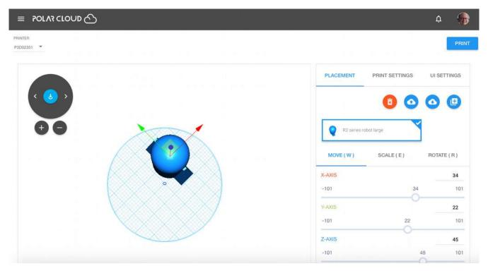
Once the file is uploaded, you can choose the printer you want to use, adjust the position of the object on the build plate, and change the print quality — all without having to go through the intermediate step of saving your file to your computer. While handy in general, this feature is perfect for those using Chromebooks!
