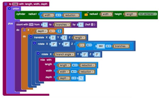
There are two things to notice in this module. First, you'll see that we don't use the Centered option for the cylinder. This makes it easy to get all the branches connected. Second, the cylinder is tapered from its previous radius at the bottom to the new one at the top — just like the branches of many real trees.
