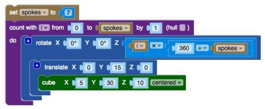
Here, we divide a circle into a number of equal sized pieces. The variable "spokes" defines how many pieces to divide the circle into. The angle of these pieces is calculated in the "360 / spokes" math block. The variable "i" counts through each piece, and you can multiply i X (360 / spokes) to get all the different orientations for the spokes. This makes the following shape.
