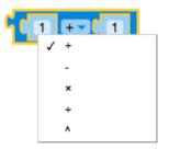
The result of this block is the combination of two numbers through either addition, subtraction, multiplication, division, or exponentiation (raising the value of the first number to the power of the second number).
