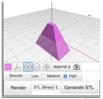
Note: Since the Taper along block is not compatible with OpenSCAD, you should use the Linear extrude block if you plan to make objects that others might edit or render using OpenSCAD themselves.
