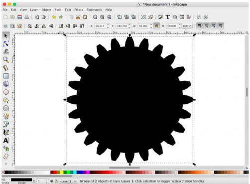
After saving the gear as an SVG file, I next used an online tool — svg2stl.com — where I uploaded the SVG file and set the extrusion depth to 5 mm. You can choose other values if you want, but this is good for now. Also, BlocksCAD lets you scale along any axis later if you wish. (We'll show how to do this in the next chapter.)
