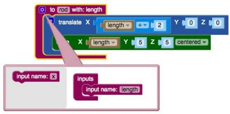
The difference from the previous examples is that the value of length applies only to applications inside the module we defined. Each time we use the same module in our program, we can have different values for the input, which is why it is called a "local variable."
