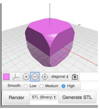
Because large parts of the sphere fall outside the shape of the cube, they don't appear in the final part. Only the areas that intersect show up in the final shape.
