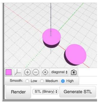
If you check the "hull" box in the block, your final shape will be the convex hull of our two cylinders.
