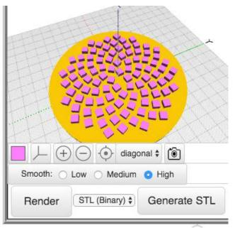
We just created one spiral in our design, but there appear to be two sets of spirals in our model, one twisting clockwise, and one twisting counter clockwise.
