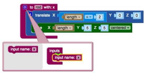
This opens a box with inputs on the right, and a block called Input name on the left with an initial variable named x. Drag this Input name block to the Inputs block and rename x with any name you wish (I used length since we used that for the rod length before).
