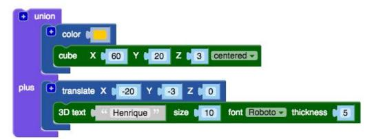
This combination of blocks gives embossed text. I used a different color for the base to make it easy to see. Of course, the color information does nothing with a single-color printer.
