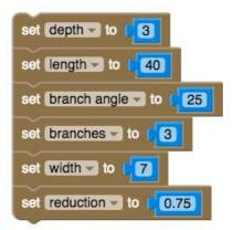
Next we define a recursive module called "tree". This module uses three local variables — the starting branch length and width and the depth (number of levels) of the tree. These three variables will have their local values changed during use of the module. All other variables will keep their global values.
