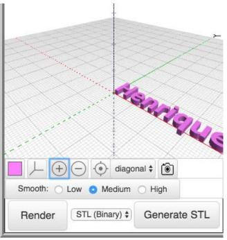
The text is drawn along the X-axis, with the lower left corner of the first character located at the origin.
