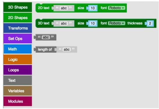
BlocksCAD supports both 2D and 3D text, and the resulting text can be used anywhere you use the original 2D and 3D graphic objects. The 3D text block looks like this:
