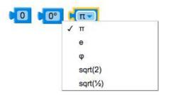
The first two items on the screen are numerical values representing (for example) a length in mm, and an angle in degrees. The third item produces the value of some commonly used constants, pi, e (the base of natural logarithms), phi (the golden mean – roughly 1.618), and the square roots of 2 and  $\frac{1}{2}$ .
