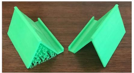
The holder on the left was printed in the normal position it would have when sitting on a desk. Because of the sloping sides, internal supports are needed to hold the sides up while they are being printed. These supports need to be removed when you are done, and they waste filament. The card holder on the right was rotated by 90° before printing. This made all the sides vertical, eliminating the need for supports. No clean up was required, no filament was wasted, and the holder printed faster.
