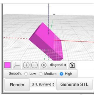
Next we draw the mirror image after setting the mirror plane to YZ.. The plane you choose is the one holding the mirror. The Mirror block provides three options for the mirror placement, the XY, XZ, and YZ planes. If you want to reflect around another plane, you can use the Rotate block before using the Mirror across block. The choice of mirroring plane is completely up to you.
