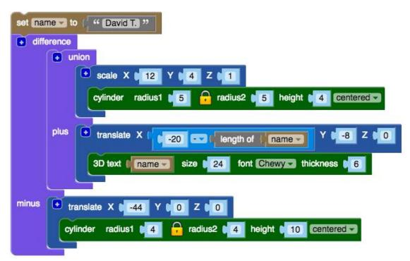
Note in the place where text is added that we offset the text along the X-axis by -20 mm minus the length of the name. The Length block produces a number equal to the number of characters in the text string. This gives us the following image when rendered.
