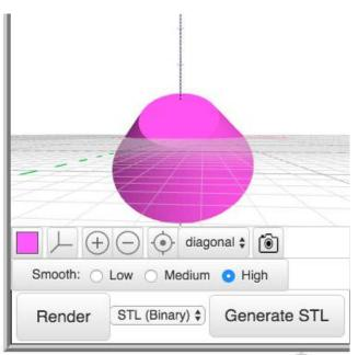
When we rotate around the Y-axis we get the cone tilted to another direction.
