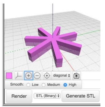
By changing the value of the number of spokes, you can make different arrangements. Notice that this object uses two variables, one for the total number of spokes, and another for the Count with block.
