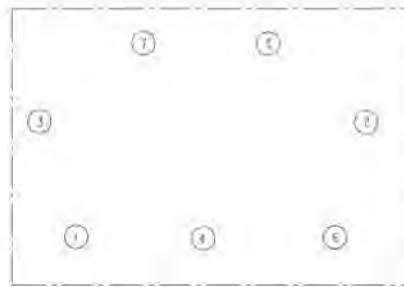
VALVE COVER TORQUE SEQUENCE
