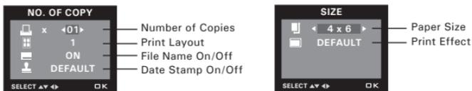
Select a setting item using the up or down button and select setting contents using the ◀ or ▶ button.
