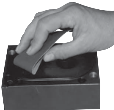
Grind if needed the functional surfaces
