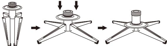
Unfold tree stand legs. Then slide the locking disc down until it snaps into place.
