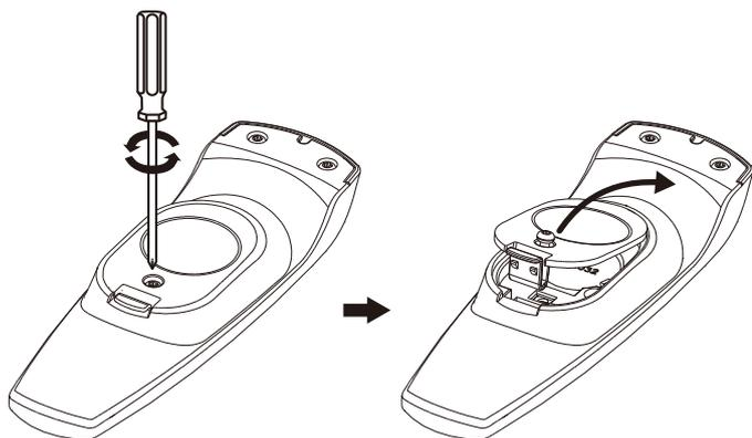
2. Replace the used battery with a new CR2032 button cell battery (not included). Make sure that the battery is installed with the correct polarity (+ and -).
