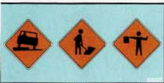
LOW SHOULDER WORKERS AHEAD FLAGGER AHEAD
