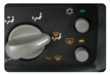
Then, with the ignition in RUN, press the defogger button (III). It may take more than one cycle to adequately clear the rear window. The defogger's first cycle will turn off after about 10 minutes, and following cycles will last about 5 minutes.
