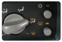
There are two modes to clear fog or frost from the windshield and side windows. Use the defog mode ()) to clear the windows and warm the passengers. Use the defrost mode () to clear fog or frost from the windshield more quickly.
