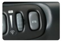
Turn this system on by pressing the ETS button, located on the left side of the instrument panel.
