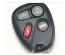
If your vehicle has this feature, you can lock and unlock your doors or unlock your trunk from about 3 feet and up to 30 feet away using the Remote Keyless Entry transmitter supplied with your vehicle. If at times you notice a decrease in range, see your Owner Manual.
