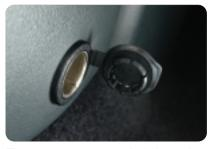
The accessory power outlet is located on the passenger side of the console. Some non-GM accessories may not be compatible with the outlet and could result in blown vehicle or adapter fuses. The fuse panel is located at the end of the instrument panel on the driver's side.
