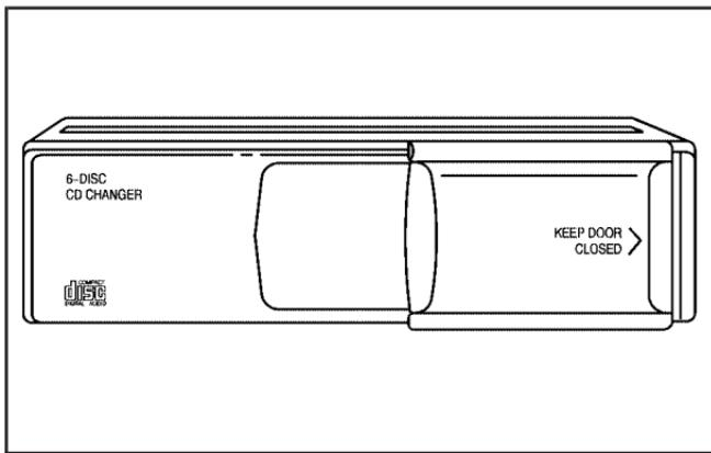
You must first load the magazine with CDs before you can play a CD. Each of the six trays holds one CD.
