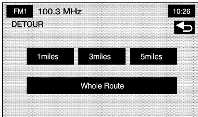
From this screen, you can select a 1 mile, 3 mile, or 5 mile detour or select to detour the whole route. After selecting the detour, the system will calculate the alternate route and the new route will display on the map screen.
