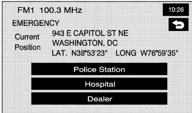
**△ Emergency:** Touch this screen button from the ENTER DESTINATION screen to access the EMERGENCY screen. The system will display the address, longitude, and latitude information of your vehicle's current position.
