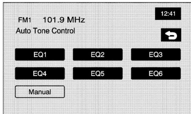
**ATC (Auto Tone Control):** The ATC feature is used to provide a choice of six different listening experiences. ATC can be used while listening to the audio system or the CD player. The audio system can store separate ATC settings for each source and preset station.
