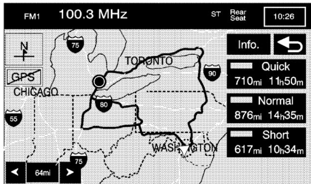
The system will calculate up to three different versions of your current route in three different colors: Quick, Normal, and Short. The routes are shown with distance to destination and estimated travel time, or select the Info screen button to access the INFO FOR 3 ROUTES screen.
