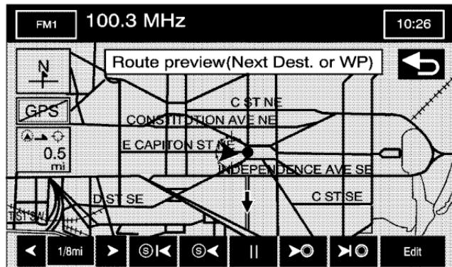
Use the screen buttons at the bottom of the navigation screen to move through the route.
