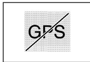
This No GPS symbol will appear in the upper right corner of the map screen when your vehicle is not receiving a Global Positioning System (GPS) satellite signal. See *Global Positioning System (GPS) on page 2-57* for more information.
