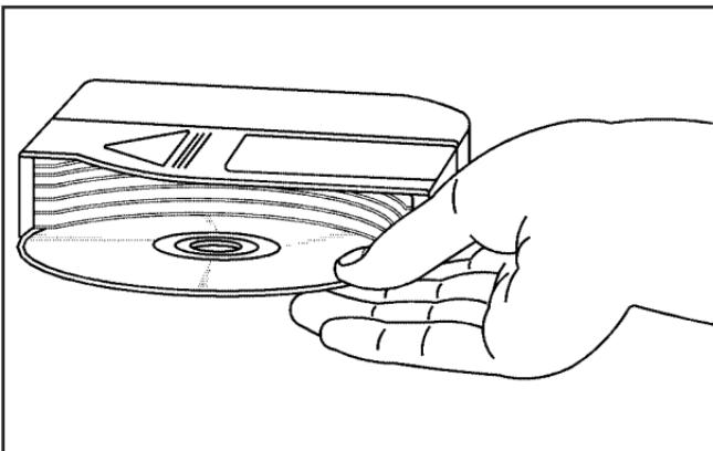
Once you have loaded the discs into the magazine, slide the CD changer door open. Push the magazine into the changer in the direction of the arrow marked on top of the magazine.
