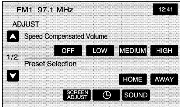
**Speed Compensated Volume (SCV):** With SCV, the audio system will adjust automatically to make up for road and wind noise as you drive, by increasing the volume as vehicle speed increases.
