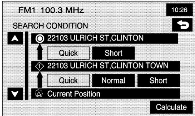
The search condition screen allows you to view your current destination and to change the planning methods between each destination. Each distance between waypoints and final destination can have an individual setting.
