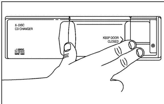
Close the door by sliding it all the way to the right. When the door is closed, the changer will begin checking for discs in the magazine. This will continue for up to one and a half minutes, depending on the number of discs loaded. You may hear noise, but this is normal. The CD changer is initializing.
