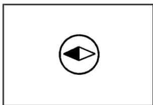
This Heading Up mode symbol indicates the map with the vehicle travel direction up.
