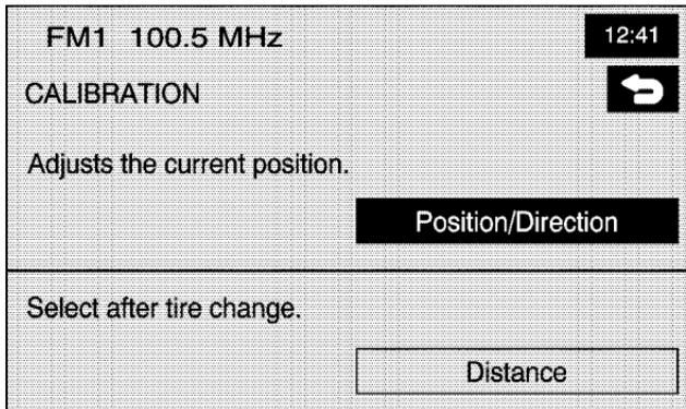
The Calibration screen, allows the adjustment of your vehicle's position or the vehicle speed signal.
