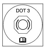
Your brake master cylinder reservoir is filled with DOT-3 brake fluid. See Engine Compartment Overview on page 346 for the location of the reservoir.
