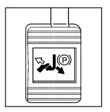
The parking brake is located to the left of the brake pedal near the driver's door. To set the parking brake, hold the regular brake pedal down with the right foot. Push down on the parking brake pedal, with the left foot.
