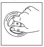
Remove the inflator kit cover by turning the center nut counterclockwise.
