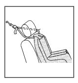
If the position you are using has a fixed headrest and you are using a dual tether, route the tether around the head restraint.
