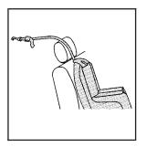
If the position you are using has a fixed headrest and you are using a single tether, route the tether over the head restraint.
