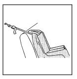
If the position you are using does not have a headrest and you are using a single tether, route the tether over the seatback.
