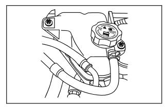
The engine coolant surge tank is located in the rear of the engine compartment. See *Engine Compartment Overview on page 5-14* for more information on location.
