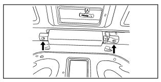
4. Remove the cover by pressing the tabs at either end with a tool.
