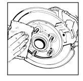
10. Remove any rust or dirt from the wheel bolts, mounting surfaces, and spare wheel.
