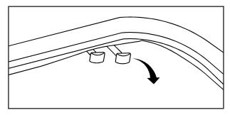
The handles that are used to lower the rear seatbacks are located on the upper edge of the trunk opening. Open the trunk. Pull the driver's side handle to open the larger side of the seatback. Pull the passenger's side handle to open the smaller side of the seatback. *Notice:* Folding a rear seat with the safety belts still fastened may cause damage to the seat or the safety belts. Always unbuckle the safety belts and return them to their normal stowed position before folding a rear seat.
