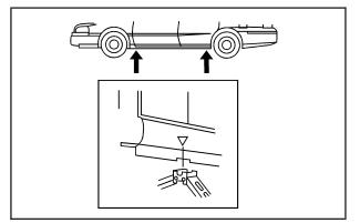
5. Position the lift head at the jack location nearest the flat tire. Make sure all of the jack lift head is touching the jacking flange under the body. Do not place the jack under a body panel. The lower body panel has an arrow to aid in locating the jacking location.
