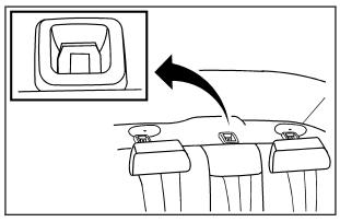
The top tether anchors are located on the rear seatback filler panel. Be sure to use an anchor located on the same side of the vehicle as the seating position where the child restraint will be placed.
