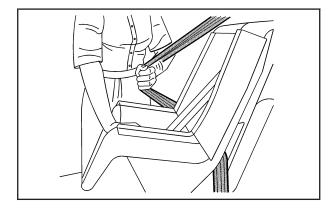
6. Pull the rest of the shoulder belt all the way out of the retractor to set the lock.
