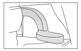
To tilt and telescope the wheel, pull down the lever. Then move the wheel up or down or back and forth to a comfortable driving position. Pull up the lever to lock the wheel in place.
