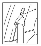
To move it down, push down the release button (A) and move the height adjuster to the desired position. You can move the height adjuster up by pushing the release button up.
