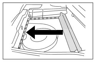
2. The trunk cargo cover must be fully closed, and the trunk must be closed before raising the hardtop.
