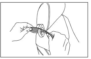
1. Remove the safety belt from the headrest-mounted guide.
