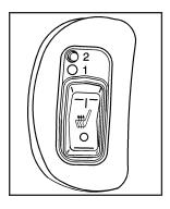
The buttons are located on the outboard side of the driver's and front passenger's seats.
