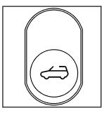
4. The hardtop switch is located on the headliner between the front reading lamps.
