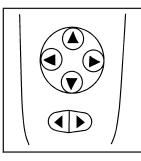
The controls for the outside power mirrors, are located on the driver's door.
