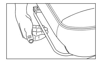
Lift the bar located under the front of the seat to unlock it. Slide the seat to where you want it and release the bar. Try to move the seat with your body to be sure the seat is locked in place.
