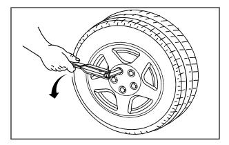
4. Use the wheel wrench to loosen all the wheel nuts. Do not remove them yet.
