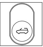
4. The hardtop switch is located on the headliner between the front reading lamps. Press and hold the switch forward to raise the hardtop. The switch must be pressed until the cycle is complete.
