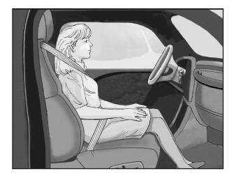
Safety belts help keep the passenger in position on the seat during vehicle maneuvers and braking, which helps the passenger sensing system maintain the passenger airbag status. See "Safety Belts" and "Child Restraints" in the Index for additional information about the importance of proper restraint use.
