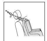
If the position you are using has a headrest or head restraint and you are using a dual tether, route the tether under the headrest or head restraint and in between the headrest or head restraint posts.
