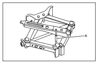
3. Place the jack over the bolt (A) on the floor, making sure it contacts the bolt as shown, and thread the jack retainer nut until it contacts the jack.
