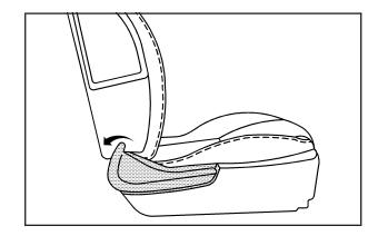
2. Pull back on the top of the recliner lever. The seatback will move forward.
