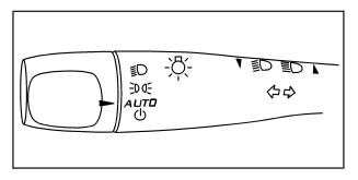
The band on the lever on the outboard side of the steering column operates the exterior lamps.
