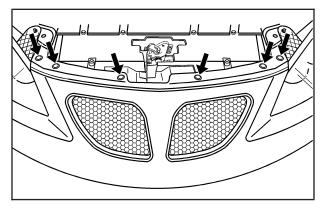
2. Loosen the front fascia by removing the plastic push pins along the top of the tie bar by prying under the fasteners with a tool. 3. Pull back the front fascia then pull the headlamp assembly forward, out of the vehicle. You need to pry the headlamp assembly away from the fender. This frees the ball stud from its retainer in the fender bracket.
