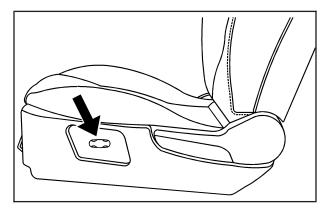
If the vehicle has a power seat, the control used to operate it is located on the outboard side of the driver's seat.
