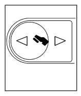
The switch used to adjust the pedals is located on the left side of the instrument panel. The adjustable pedal feature is meant to be used with the adjustable seat and adjustable steering wheel controls to reach a safe and comfortable position.
