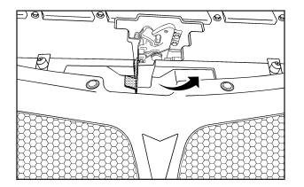
2. Then go to the front of the vehicle and push the secondary hood release lever to the right.
