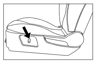
To adjust a power lift seat, press the top or bottom of the power lift seat switch to raise or lower the seat.
