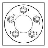
14. Tighten the wheel nuts firmly in a crisscross sequence, as shown, with the wheel wrench.
