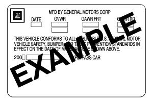
A vehicle specific Certification label, found on the rear edge of the driver's door, tells you the gross weight capacity of your vehicle, called the Gross Vehicle Weight Rating (GVWR). The GVWR includes the weight of the vehicle, all occupants, fuel and cargo. Never exceed the GVWR for your vehicle, or the Gross Axle Weight Rating (GAWR) for either the front or rear axle.
