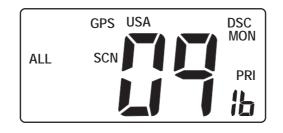
The noisy channel is now removed and the 7-channels/second scanning of all channels can continue. Turning the radio OFF/ON again restores all the channels back to original condition. There is no memory of deleted channels.
