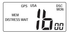
The Coast Guard is the only agency allowed to ACKNOWLEDGE (ACK) a DISTRESS call. An Individual vessel's DSC radio will not respond automatically with an ACK. When an ACK is received, the radio distress mode is automatically cancelled & voice communication is on CH16.
