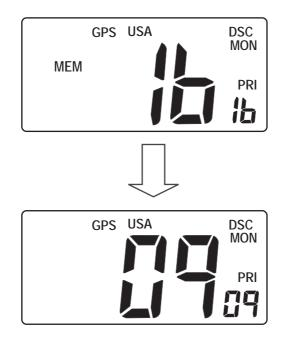
A quick press of the 16/9 key immediately selects the priority channel (16 or 09) with HIGH Tx power. Another press selects "last used" channel. This action does not over-ride the HI/LO power function, except for the priority channel itself.
