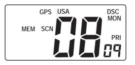
To cancel scanning press the SCAN key again or the 16/9 key. PTT exits the scan mode at the last channel display.
