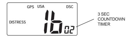
If the DISTRESS key is held down until the timer expires (0 seconds), the DSC DISTRESS message is transmitted at 25 watts. The radio switches to channel 70 & Tx will come on for about 1-2 seconds. The DSC message is transmitted 5 times without a break. This message contains your MMSID, LL position and UTC time acuired from your GPS navigator. The "DISTRESS" annunciator is displayed during the transmission.
