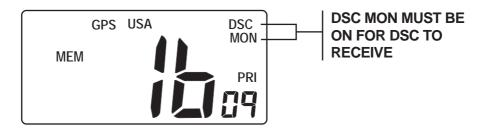
Under normal conditions, you will not even notice this CH70 monitoring activity, except that all scanning modes will be somewhat slower. If you wish "fastest possible channel scanning", just turn the DSC Monitor Off. DSC operation is OFF and the radio will not receive any calls. DSC is disabled.
