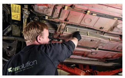
**Above** Fresh fluid changes are essential every twelve months, regardless of mileage, to avoid oil and brake fluid pipework corroding from the inside out
