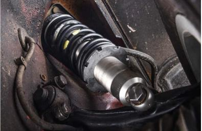
The application-specific part was easy enough to come by through Porsche, but the bolts holding the kit in place are no longer serviced. Danny enlisted the help of a trusted metal specialist when it came to identifying the properties of the original bolts, a move that enabled him to have suitable replacement parts made to order. In his own words, "engineering ability is unquestionably more important than parts availability when it comes to keeping a 959 on the road in the present day."
