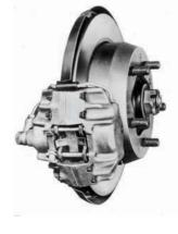
356C models, launched in 1963, and were so good that they continued in production, virtually unchanged, when the new 901 (which became the 911) was released. In fact, the only difference between the 356C and 901/911 disc brakes was a slight increase in diameter of the front discs (to 282mm) on the otherwise all-new model.
