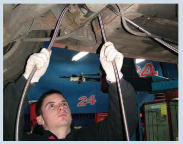
In both 924 and 944 the fuel and brake lines pass between the rear end of the floorpan and the transverse tube housing the torsion-bar road springs.
