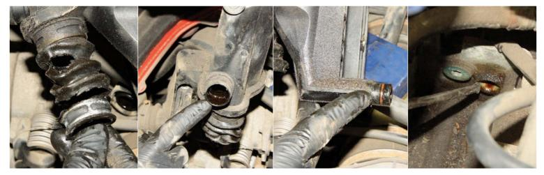
It's possible that a perished 'bellows' may be the primary cause of your air/oil separator problems, but plainly there's very little point in replacing that alone, since realistically you have to remove the separator to do so. Second photo shows more clearly the lower of the two vacuum ports on the side of the separator body, and the third the stub at its lowest point, which you had to ease out of the corresponding hole on the side of the crankcase (far right). Easy when you can see what's what
