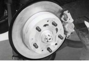
cast-iron disc on which acted a cast-iron caliper containing two pistons the costly to produce annular brakes featured four-piston calipers designed to automatically align the pads and return them to the correct position after use. The other unique feature on the Porsche-developed brakes was the inclusion of the drum-type handbrake at the rear.
