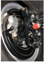
The annular disc brake is a fascinating design, with the caliper mounted 'inside' the disc. This allowed a largerdiameter disc to be used. However, the 356C (and the first 911) used this more conventional disc (right), which followed Dunlop's original layout, with an external caliper. A drum was located within the rear brake disc to serve as the emergency handbrake
