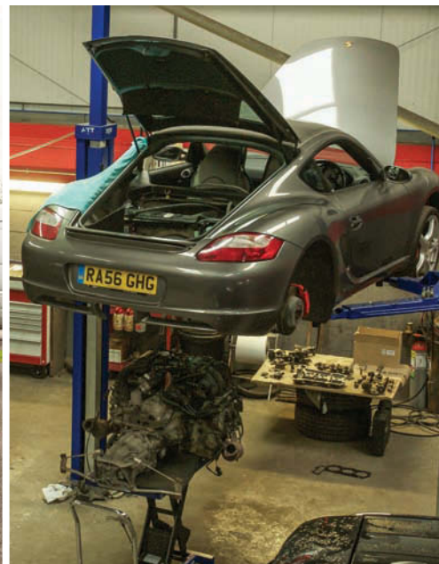
Cayman on the ramp, with engine dropped out for rebuild, bore scoring the culprit. Left: Courtesy cars are two very smart current gen Golf GTDs
