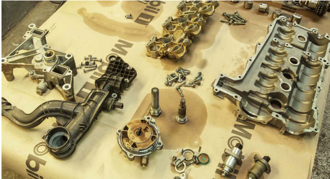
Steve Bull carries out his fair share of engine rebuilds on modern Porsches. Worst offender is the gen 1 997, largely for bore scoring
