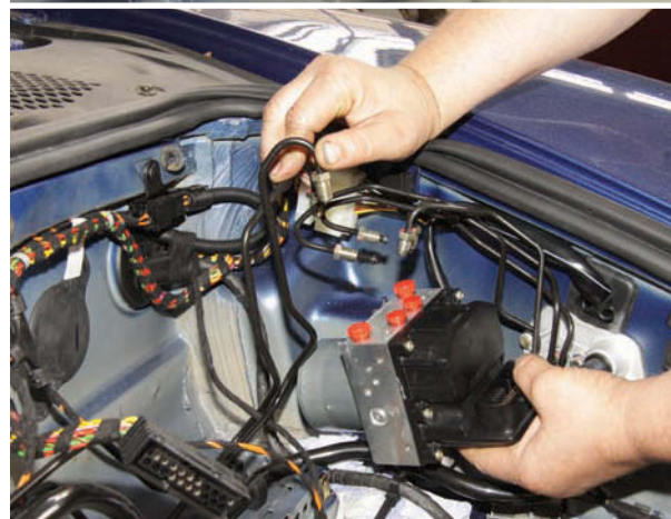
Even the Boxster's replacement discs (top) were 'blued' by the car's spontaneous application of its brakes – but nowhere near as badly as the originals had been. Brake master cylinder was found to be from a Vauxhall – and replaced – and a new servo fitted, too. Next step was a replacement ABS pump (above), and finally what Porsche calls a 'venturi tube' in the vacuum line to the manifold
