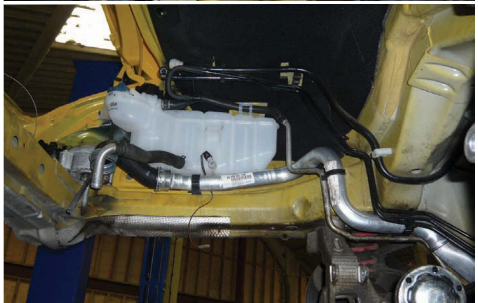
Photographs supplied by PIE show work in progress on a customer's 997 GT3 – although the job was prompted by a clutch issue rather than a cooling-system problem. As standard (and on the 997 Turbo, too), pipe stubs are glued in to thermostat housing, but PIE has them securely TIG-welded (top). Middle photo shows thermostat housing back on the engine, and the latter installed in the vehicle. The same car benefited from preventive fitment of a new coolant expansion tank – they can crack
