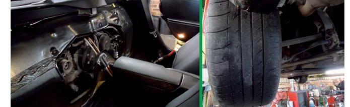
Left: So that's where the engine is! Interior panel removed to change drive belt. Rear Michelins have covered 17,000-miles, with another 5000 miles of life left in them
