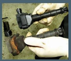
All 986–997 spark plugs are fired by their own individual ignition coils, which because of the harsh environment in which they work – especially in the mid-engined Boxster and Cayman – have a relatively short life. They are a little awkward to replace, though, so it's probably best to have all six done at once rather than wait until the next one fails – as it surely will...
