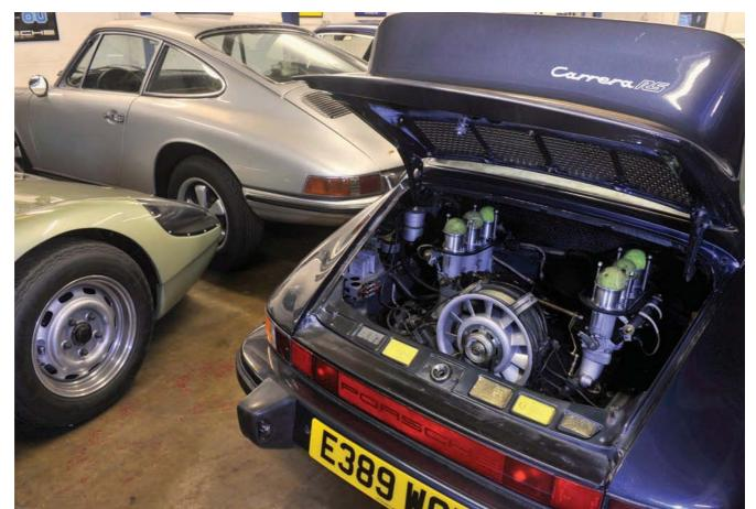
Right: Anyone for tennis? Carrera 3.2 with ducktail and fuel injection throttle bodies. Together with a bespoke ECU, this mod liberates an easy 20bhp
