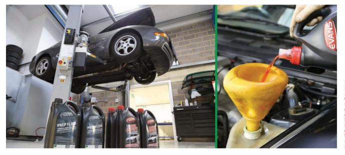
Ken's 968 being replenished with Evans Waterless Coolant. Top end rebuild revealed extent of water damage. Head gasket had nearly rotted through. Evans coolant extends boiling point and minimises pressure in the system
