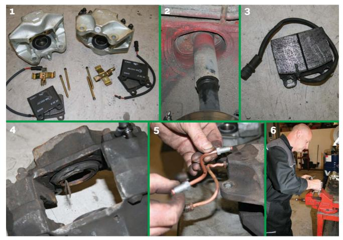
bits needed. After much 'phoning around he located a pair of original ATE remanufactured calipers, but the piping was not readily available. No problem though, said he, because he could make them up in the workshop. (SVP builds race and rally cars from scratch and so is adept at manufacturing bespoke brake systems and, indeed, electrical wiring looms.)
