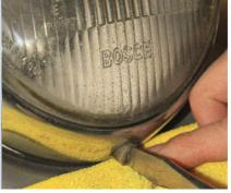
Standard headlamp glass has a chromeplated trim, and perhaps a body-coloured trim over that (far left and middle). If the latter, undo the fixing screw at the 'six o'clock' position, and then in both cases the further larger screw securing the entire lamp assembly to the recess within the front wing. Cloth protects paintwork
