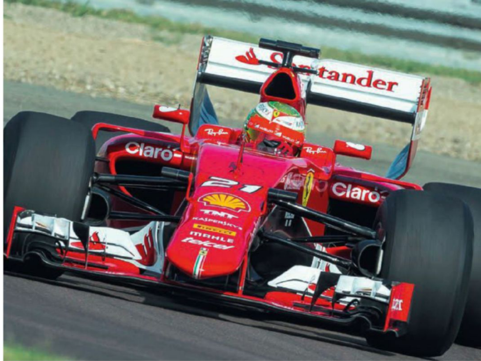
A 2015 Ferrari 'mule car', fitted with an aero pack to simulate 2017 downforce levels, tests the new Pirelli tyres
