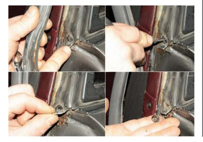
Even then the glass was surprisingly reluctant to start moving, such was the quantity of sealant that had previously been used, presumably to try to stop a leak. Trick is to start at one corner, then the other, all the time trying to use firm but gentle force, rather than localised pressure. Once it was out it was immediately obvious that the visible rust at the base of each pillar had been just the start
