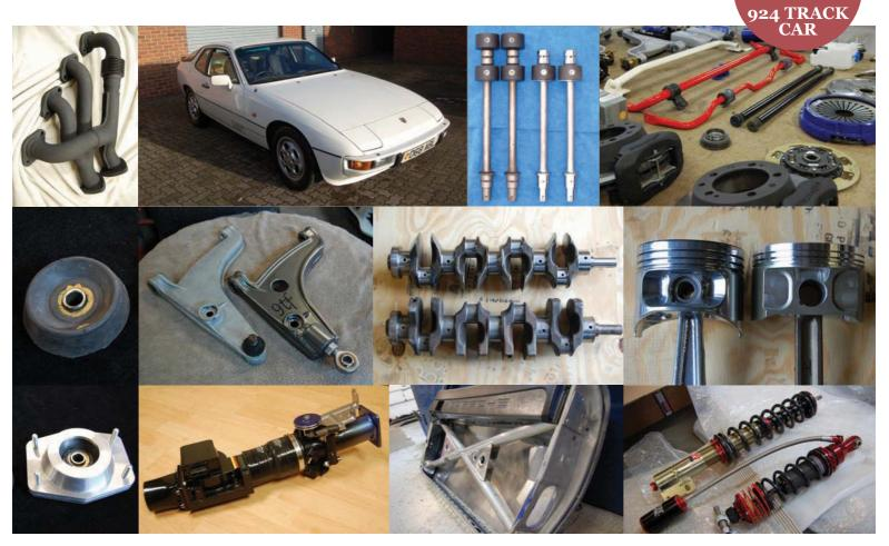
Just some of the parts from this epic build. Starting point was a nice, clean 924S. Lightweight balance shafts make for an eager engine as does lightened, knifeedged crank and lightweight pistons and rods. Note clever, adjustable suspension arms, plus lightweight doors and fabulous Intrax suspension
