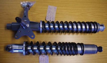
stiffen up before the damper closes completely; because, if you start to run springs which are too soft, obviously there's nothing to stop the wheel going up and you can start to bottom out; if they're nice and soft and you're going over speed bumps, let's say, the wheel will just come straight up, and then anything can happen.
