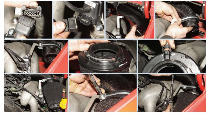
There is a new moulded intake pipe that sits between the air filter and the throttle body, fixed to the MAP sensor's bracket with a large rubber-lined 'P'-clip; as ever in such circumstances, leave all fixings just a little loose until everything is in position and correctly aligned. Don't forget simple plug-in wiring connection to the temperature sensor; it's ĥard to get at when filter is located on the new pipe. All wiring is supplied, and ready - almost literally – to plug and play
