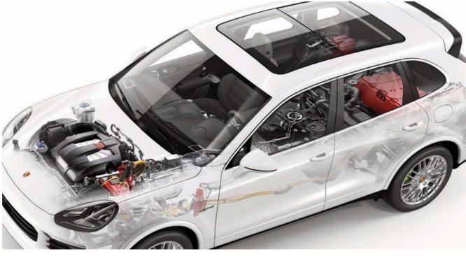
upgrades were applied across the range including a new, eight-speed Tiptronic S automatic gearbox, auto start stop function, improved thermal management of the engine and transmission, and a "smart" alternator that switched off when charge is not needed, thus reducing engine load.
