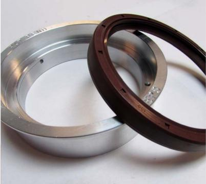
Rear Main Bearing Seal and Housing
