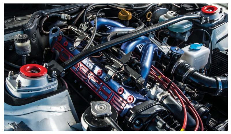
system was given a Zircotec coating to keep the heat in and under bonnet temps down. The inlet manifold was shortened for a straighter flow of air from the standard throttle body and internally polished to speed up the airflow into the engine.
