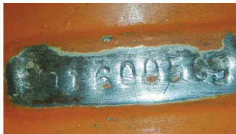
Stretch marks in metal, and insufficient characters, suggest this '1976' chassis number to be a fake
