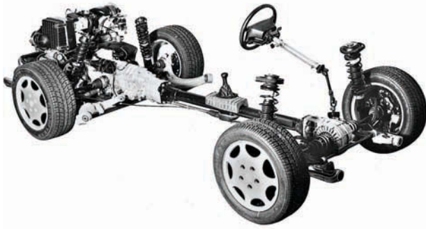
Above: The bare bones of the 964-series Carrera 4 displaying the rigid torque tube that connected the front differential to the nose of the transmission
