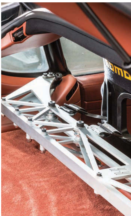
Above: Brey Krause rear strut brace and harness mount is a nice interior touch. Momo bucket and four-point harness keep driver firmly strapped in
