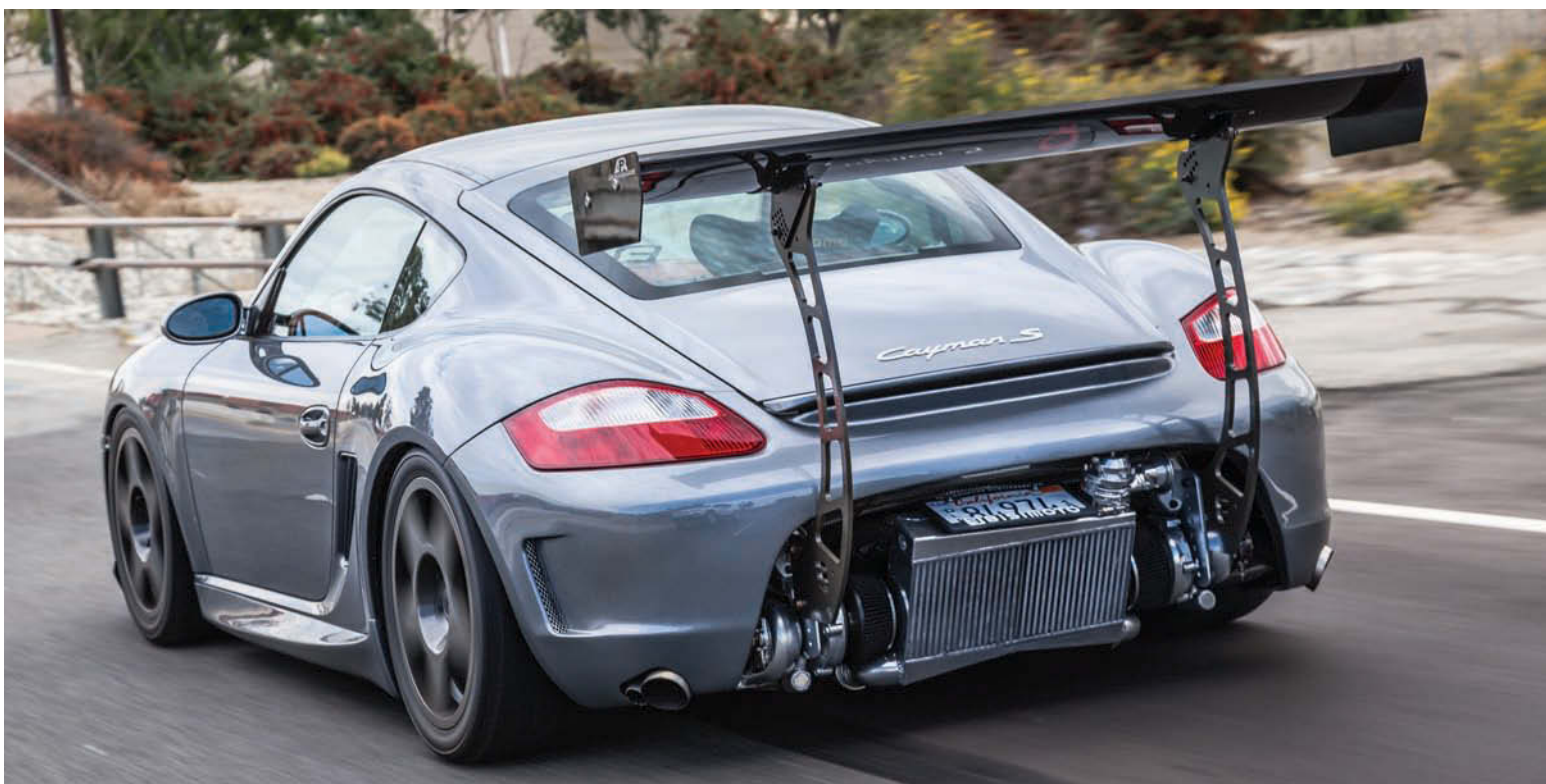
Rear carbon wing is removable for more of a sleeper look, although there's no getting away from exposed turbos and intercooler, which rather give the game away
