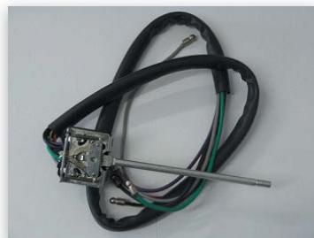
Turn Signal Switch for 356A (1955-1959) models 644.631.301.00
