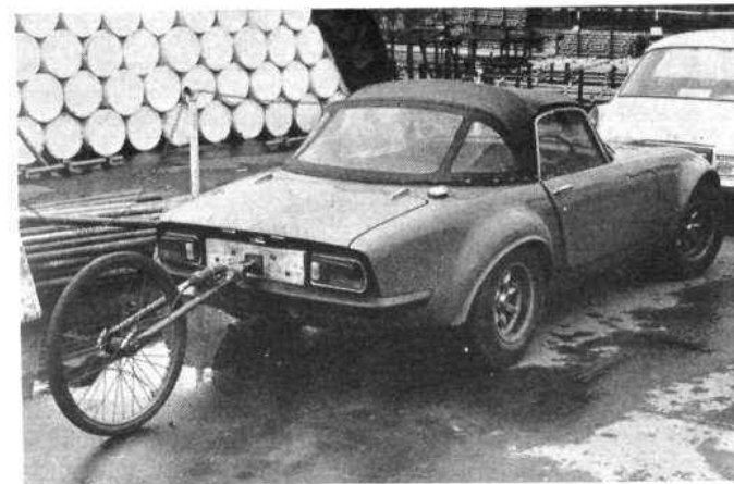
NO! J.W. has not just run over an unfortunate cyclist. The Elan-BDA pictured with the fifth wheel timing device rigged up. Unfortunately during the test runs the car suffered from a cam seizing in its carrier and so we were not able to obtain what surely would have been some of our most impressive acceleration figures ever.
