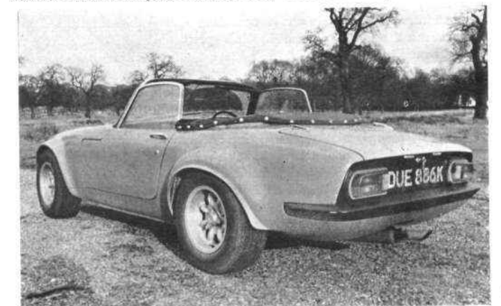
THE ELAN-BDA looked impressive with its fat tyres on some excellent Minilite rims and the bulging wheel arches to accommodate them.
