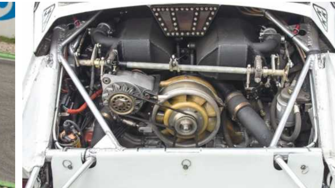
Above and left 911 underpinnings are plain to see; in a first for the 911, the 935/78's powerful 3.2-litre engine found itself loaded with water-cooled cylinder heads
