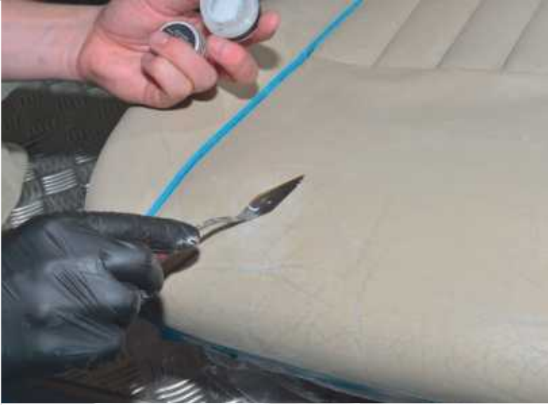
Above and left After carefully cleaning and sanding the damaged leather, Simon painstakingly filled cracks, nicks and rips with flexible filler designed to withstand heavy traffic; colour-matching faded leather can be tricky, but our man Walters came up trumps with the perfect pigment
