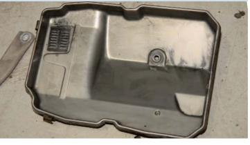
It should be a very simple matter to degrease and clean the sump pan, both inside and out, but note this internal magnet (top row, middle photo), designed to trap ferrous particles within the fluid – so don't be too alarmed if you see any; that's entirely normal. (How many are too many? You'll probably have to use your own judgement for that, but seek professional advice if both the magnet and/or the fluid seem especially contaminated.) Discard the old gasket
