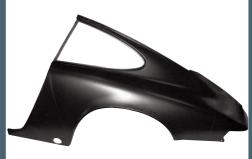
The huge range of top-quality repair panels from Dansk has been joined by this complex fuel-filler surround (left), and what might be termed a partial rear wing, designed to be cut into smaller sections, as necessary
