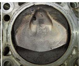
Three piston crowns from the same 23,000-mile, 2010-model 997 Turbo show the washing (or in one case not) effect of markedly different injector spray patterns, argues Ellisdon. Combine this misdirected and possibly excessive flow with reduced lubricity and perhaps increased water content of ethanol fuels, and you have the perfect storm
