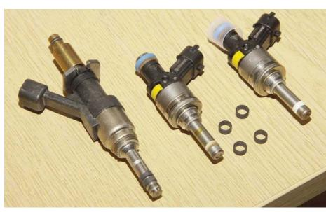
From right to left: new 997 injector, showing white Teflon stem seal; a used injector from the affected engine, showing discolouring, and staining of stem; BMW injector, with two grey graphite-based seals
