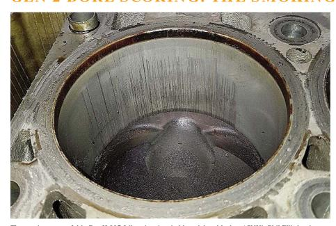
The precise cause of this Gen II 997 failure is – inevitably – debatable, but ASNU's Phil Ellisdon is convinced it's down to something as small and seemingly insignificant as a fuel-injector stem seal
