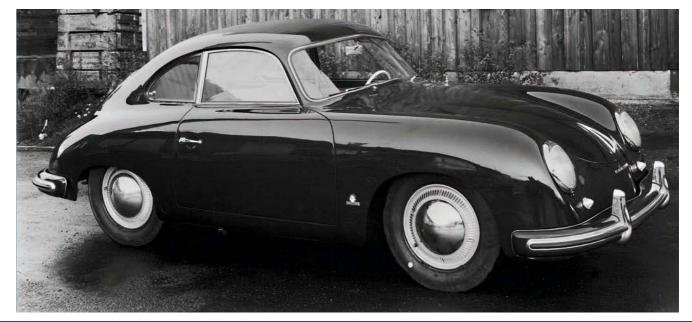
A styling tidy up in 1952 saw the twopiece bent windscreen replaced with a single curved screen. The rear cabin also gained a folding seat
