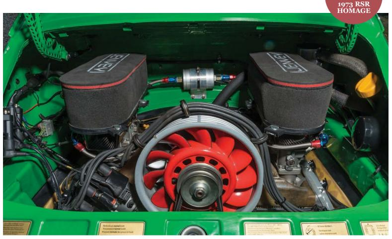
Above: 3.6-litre 964 engine produces 340bhp and 260lb ft of torque. Jenvey throttle bodies and Motec ECU smooth out the wild nature of the RSR 'Sprint' cams sprayed the whole lot Viper Green.
