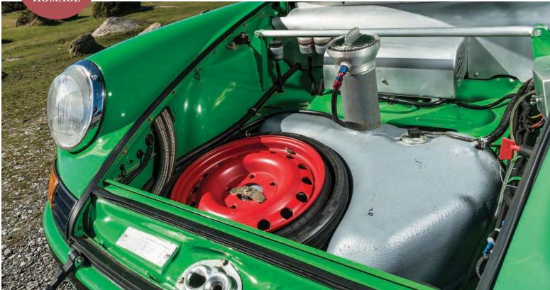
Above: Attention to detail is obvious when you open the bonnet, with aluminium shrouding covering the wiring. Note the centre-fill fuel tank conversion
