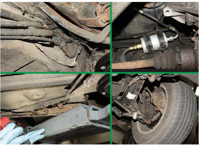
smooth as it has always been – and that despite what is fairly obviously a weakened right-hand engine mount. (Certainly the large-diameter coolant hose is far closer to the chassis rail than it is in the 924S. That's the usual giveaway of that problem in these cars. And when I later replaced the undertray, the steering-pump pulley was plainly going to start cutting into it. Needless to say, I took the undertray off again until such time as I can find and fit another engine mount.)
