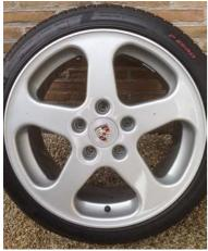
Genuine Ruf wheel set for Porsche 993 Ruf wheels (complete set of 4) for Porsche 993 including tyres Pirelli P Zero. Front: wheels 8.5 J x 18 H2 ET58, tyres 225/40 ZR 18 N4 DOT 0910; rear: wheels 10 J x 18 H2 ET66, tyres 285/30 ZR 18 N4 DOT 3607. Wheels are in perfect condition, no damage at all, tyres are perfect with 7mm profile, centre caps not included, fits C2, C4, Targa, S, 4S, RS, Turbo. Tel: 32 475 723939. Email: guysteen68@gmail.com (Belgium) £2400/€2750 P0717/037
