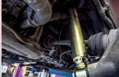
Front struts are paired with fullyadjustable rear damper units. Plated finish is attractive and practical at the same time
