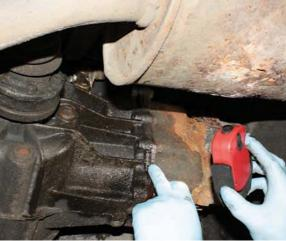
At the rear Henry noted the leaking transmission (left), suggesting the source will probably be the selector-shaft seals. Also the deteriorating anti-roll-bar rubbers (far left), but they will be easy enough to fix. Unsurprisingly, the whole of the underside is showing signs of surface corrosion, but no major problems so far
