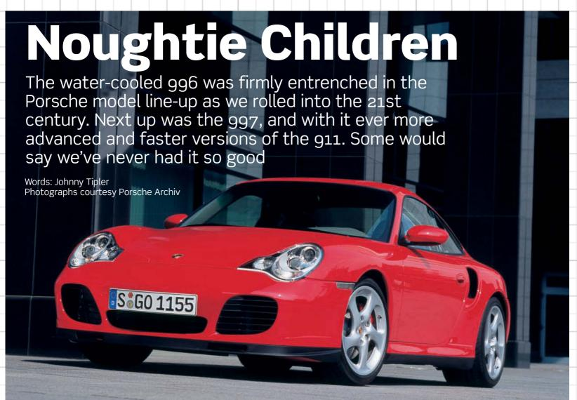
he new Millennium opened with a bang: Porsche's first new model for the new century was the 996 Turbo, unveiled at the 1999 Frankfurt Salon and prowling the streets by Spring 2000. Re-introduced after a two-year hiatus (following the demise of the 993 version), the water-cooled 996 Turbo was constructed on the broader C4 body and featured a 24-valve 420bhp flat-six with double valve-springs, twin-turbos and intercooler, with reinforced A-pillars and rear bodywork widened by 65mm to
