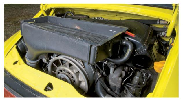
The DP Motorsport 3.3-litre Turbo S engine is dominated by a huge intercooler. Power is a lazy 36obhp, but adjustable boost control means it can be tweaked to over 40obhp
