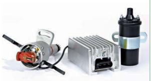
times, and the €1550 (£1330) price for all models includes converting the existing distributor to a completely electronic function. The distributor obviously has to be sent into the company, and once modified serves only to actuate the ignition module, the job of the ignition advance being taken over by the ignition module itself.
