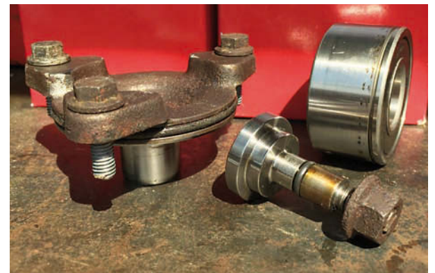
Whether or not this early double-row IMS bearing has the right central spigot to allow an after-market set-up to be converted back to standard specification is uncertain, but even the possibility that it does shows the value of stockpiling old parts for a rainy day
