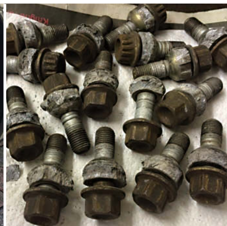
Might your outwardly smart 997 wheels (or 996, Boxster, Cayman rims etc) be concealing disastrously corroded securing bolts, like these? In truth, it's the conical collars that are corroded, not the bolts themselves, but the result will be much the same, suggests Darren Collins. You have been warned!
