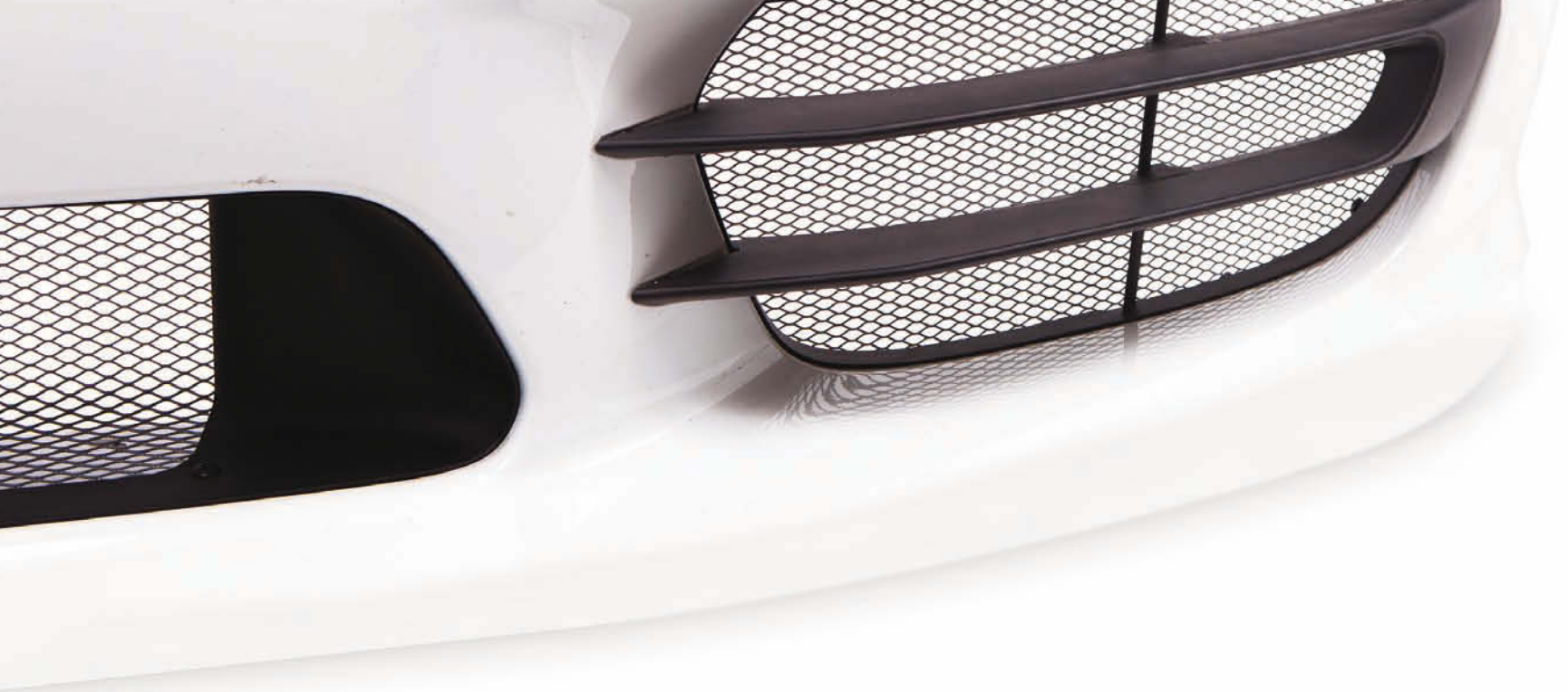
RADIATOR PROTECTION GRILL SCREENS
