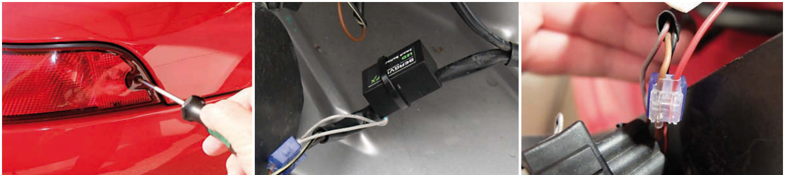
Clever little ‘ballast’ device (middle photo) from Norwegian Porsche electronics specialist Bergvill is designed to allow earlier Porsches with cruise-control also to run LED brake and tail-light bulbs. It fits neatly behind one of the rear light units – and only one unit per car is required. ‘Scotchlok’-style connectors permit quick and easy wiring
